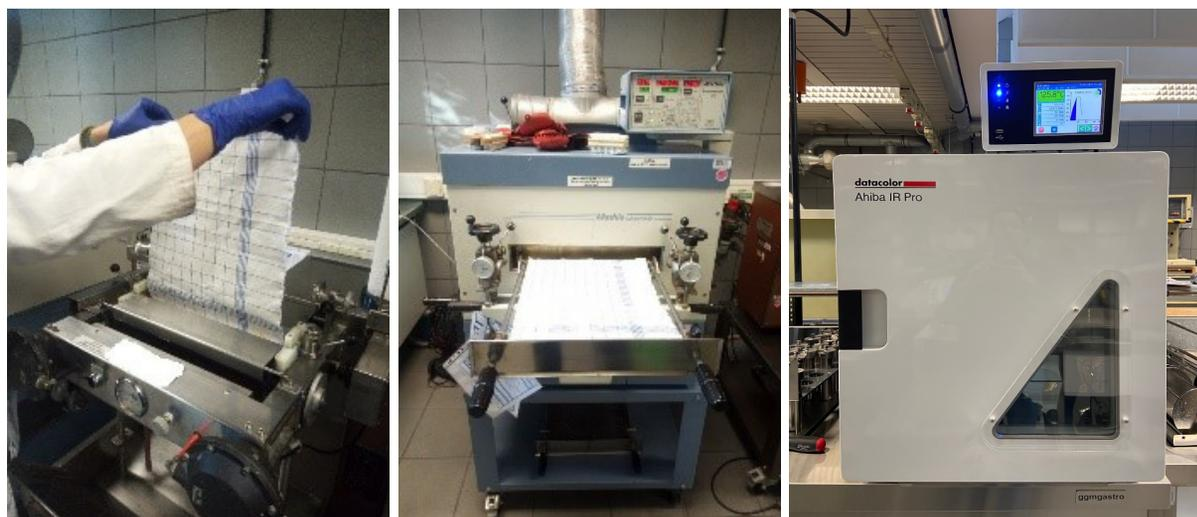
Figure 2 – Photographs of used devices – padding, drying, dyeing (from left to right)
